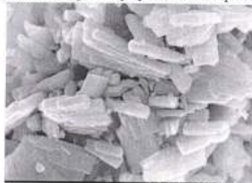
Fig. 4 SEM image of as-prepared CdSe nanoparticles
